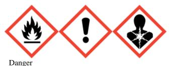
H226-Flammable liquid and vapour. H319-Causes serious eye irritation. H315-Causes skin irritation. H372-Causes damage to organs through prolonged or repeated exposure (central nervous system). H412-Harmful to aquatic life with long lasting effects.
